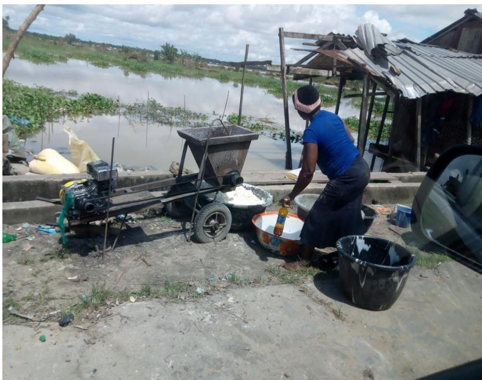
Fig 4. Grinding machine with a woman holding red oil to make yellow garri.
