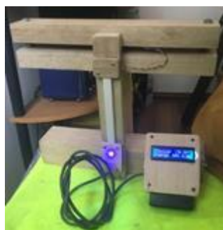
Figure 14. Functional device to measure the force and flexion of the foot. Own elaboration.
